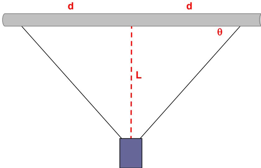
Once the two spring scales read the same value for each trial, you were able to determine the value of side **L** in the above right triangle by subtracting the height of the suspended mass above the table from the distance between the top of the table and the height of the horizontal supporting bar. The value of **d** was calculated by dividing the distance separating the two clamps in half.
