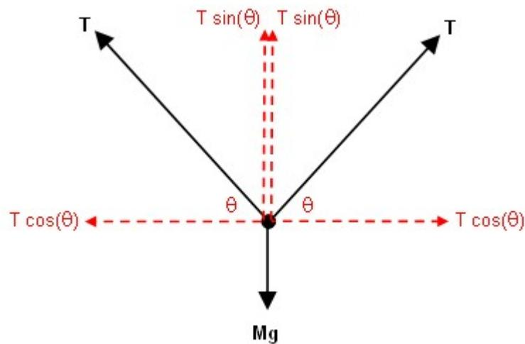
In fact we could construct yet a third diagram only showing the components of the tensions and the weight.
